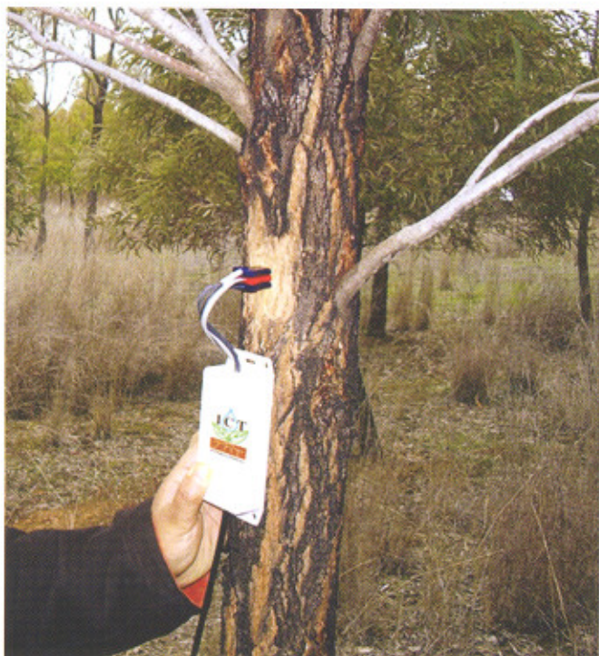
The hand-held Sapflow device being used in a tree to determine the amount of water it consumes.
